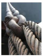
Abrasive wear occurs on the inside and outside of wire ropes when strands inside the rope move & rub against each other. The outside of the cable accumulates dirt and contaminants from sheaves and drums which erodes the outer wires and strands.
